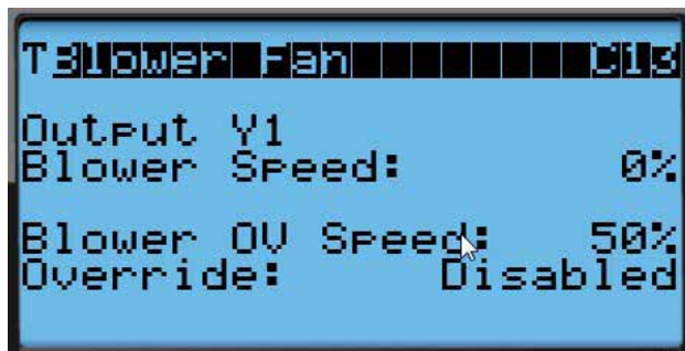
FIGURE 15 Putting Blower Output into Override Mode
