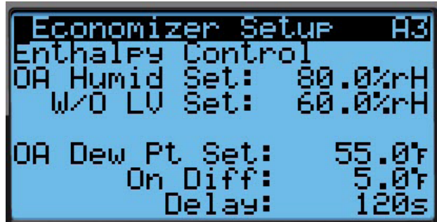
FIGURE 44 Economizer Setup – TempHum Control
