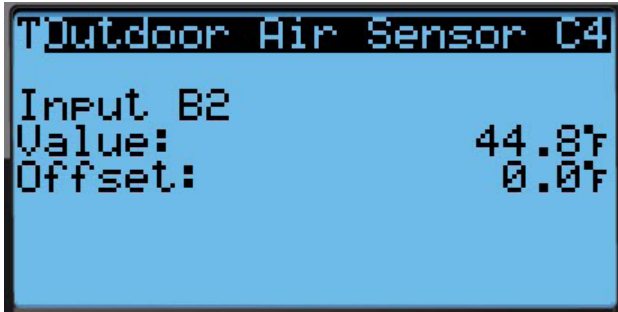
FIGURE 38 Outdoor Air Sensor
