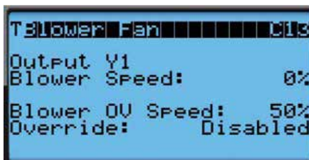
FIGURE 16 Putting Blower Output into Override Mode
