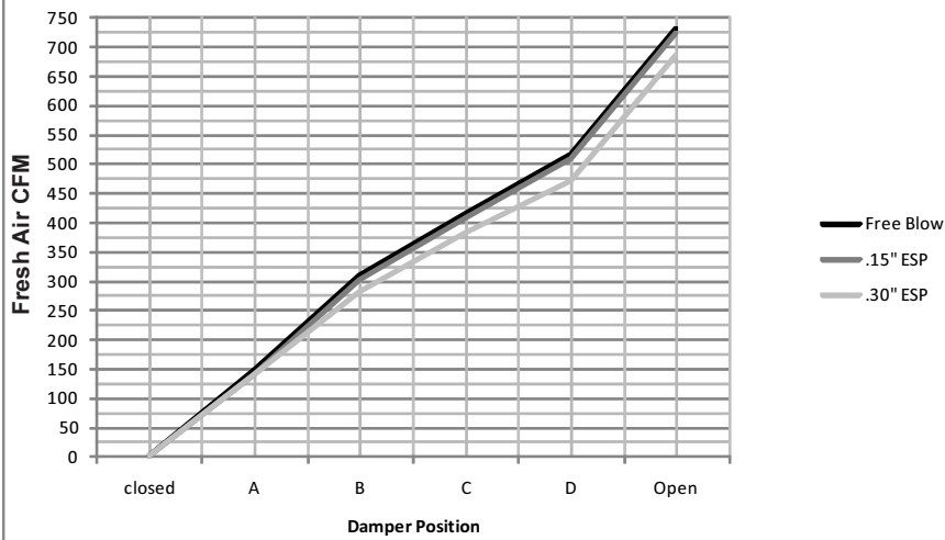
W24G CRV Airflow Versus Position - High Speed
