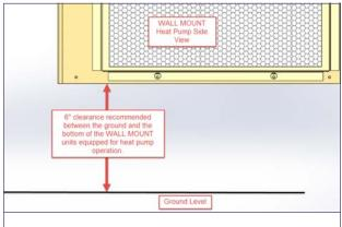
6" clearance is recommended under WALL-MOUNT heat pump products to allow proper defrost water drainage.
