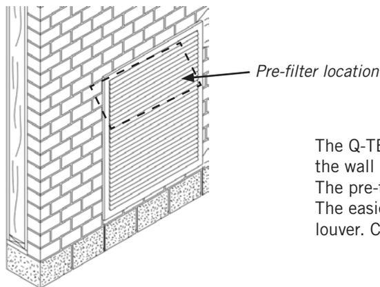
The Q-TEC will have a permanent pre-filter installed inside the wall sleeve if air intake vent options are inside the unit. The pre-filter must be inspected and cleaned when necessary. The easiest way to remove the pre-filter is through the outdoor louver. Clean the pre-filter with soapy water.
